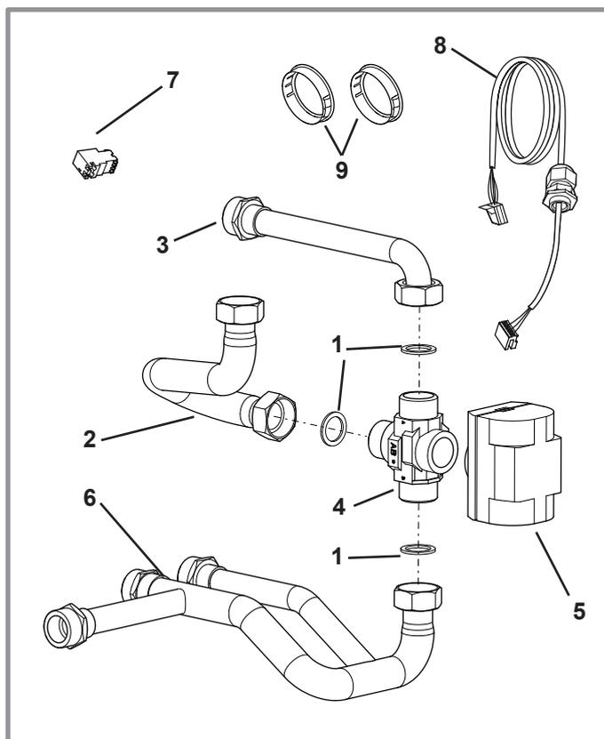
figure 12 - Spare parts Boiler connection kit
