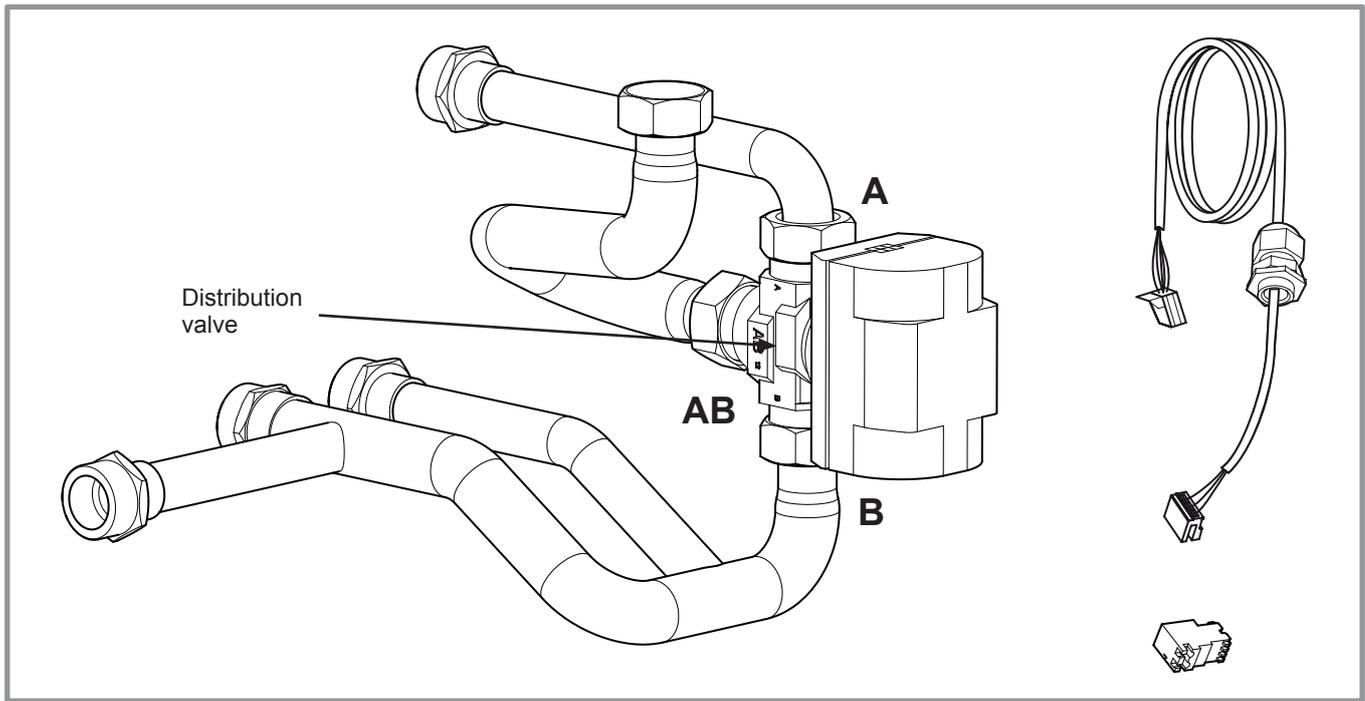
figure 4 - Boiler connection kit
