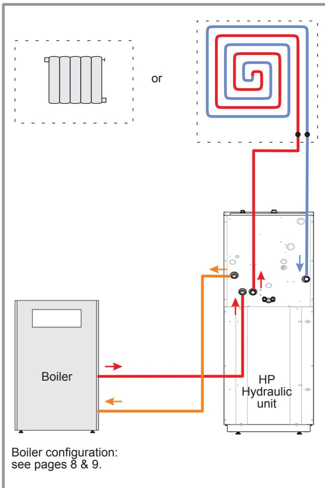
*figure 3 - Overall hydraulic layout*
