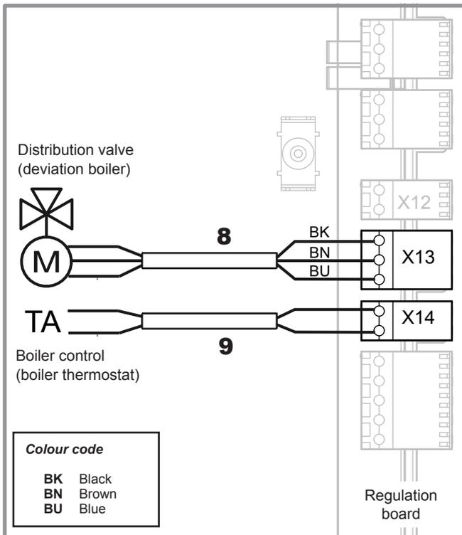
figure 9 - Electrical wiring
