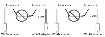
(3) Group connection of indoor units with WLAN adapter cable.
