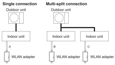
A, B, and C are adapter cables attached to this product.
